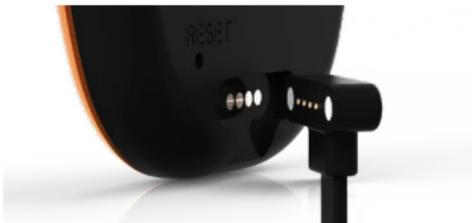
3. **When the Vario LS is OFF** and connected to the power source the display shows the message "**CHRG**". When the battery is fully charged the display shows the message "**FULL**". If the Vario LS detects some problem with the battery the display shows the message "BAD", this can be caused by trying to charge the instrument in an excessively hot environment.
