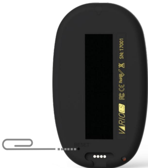
**2. Put the Vario LS into “fail safe” mode:** keep the Power/Menu button pressed, while pressing the reset button. Keep the Power/Menu button pressed until a counter is displayed on the screen. After the counter ends the Vario LS should display **“SAFE”** text on the graphic area. The firmware can now be installed by using manual update (chapter 4), or, exit the “fail safe mode”, pressing the reset button again.
