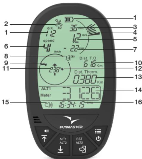
**Battery level** - This indicates the battery level of your instrument.
