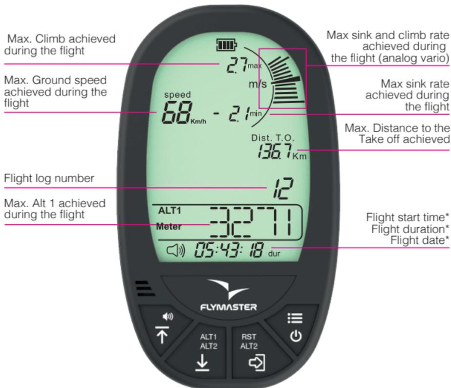
\* The flight start time, flight duration and flight date are shown in sequence
