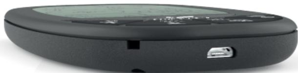
3. **When the GPS LS is OFF** and connected to the power source the display shows the message **"CHRG"**. When the battery is fully charged the display shows the message **"FULL"**. In both cases the battery icon will show an animation of the battery charging and status. If the GPS LS detects some problem with the battery the display shows the message **"BAD"**, this can be caused by trying to charge the instrument in an excessively hot environment, or a damaged battery.
