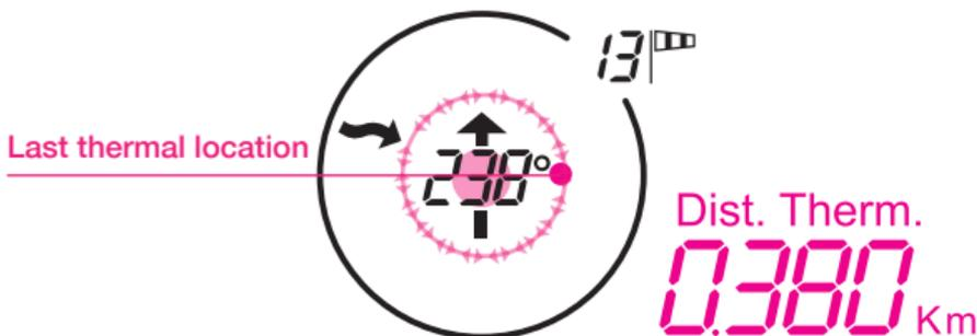
**Last thermal** - The moving ball (last thermal location) will rotate in both directions indicating **the location of the last thermal**, considering the center of the circle is your position. The data field "Dist. Therm." indicates the distance from the thermal.
