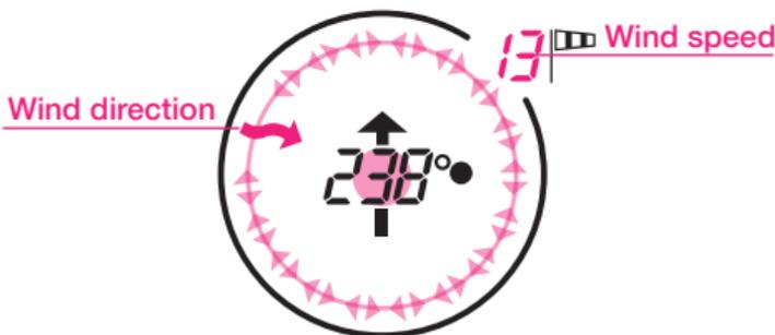
**Wind indicator** - The outside arrow (wind direction) will rotate in both directions indicating **from where the wind is blowing**, considering the center of the circle is your position. The upper right data indicates the wind speed.
