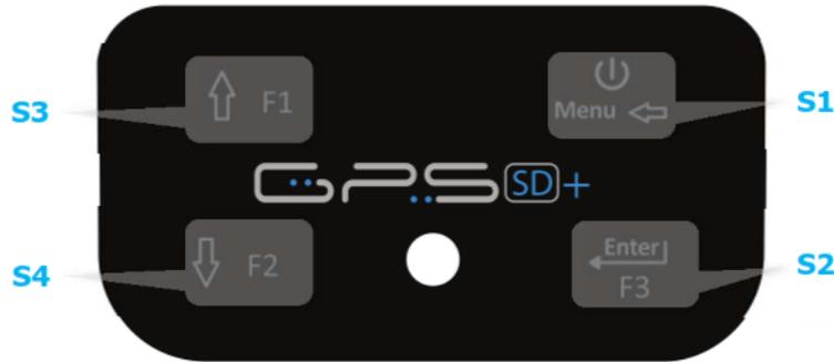
Figure 1.2: GPS SD+ keypad
