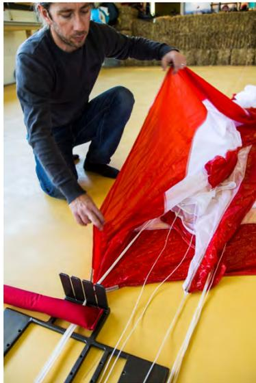
Pic. 54 Go along the bottom edge from the middle line to the first line
